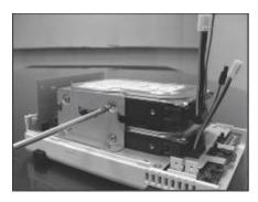
8. Connect the HDD Data Cables and HDD Power Cables to the motherboard correctly according to the disk number.
