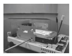
6. Place the other hard disk in the HDD bay. This disk will be disk No.2 (disk#2).
