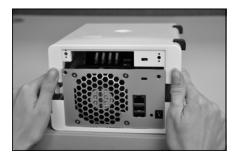
4. Place the hard disk connected with the shorter HDD Data Cable in the HDD bay. It will be disk No.1 (disk#1).
