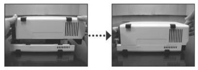
10. Fix the case with the 2 case screws provided.
