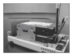
7. Fix disk#2 with the other 4 HDD screws provided.
