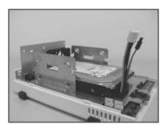
5. Fix disk#1 with the 4 HDD screws provided.
