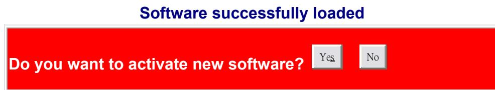
Press “yes” then you get new code to execute. **However, after activating the new code,** it is better to press **“reset button”** at front panel so that the new default setting will be also updated, because different version code is sometimes with different initial default setting.
