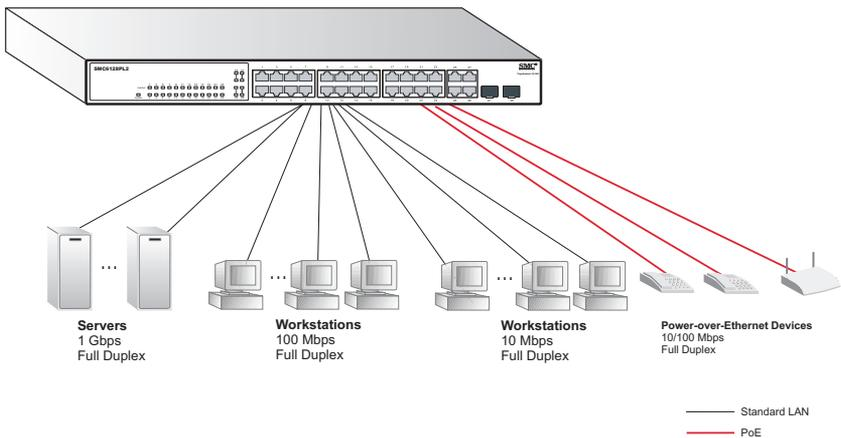
**Figure 2-2 Collapsed Backbone**
