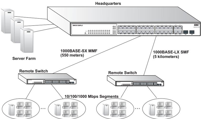
**Figure 2-4 Remote Connection with Fiber Cable**
