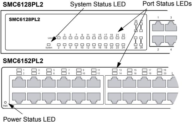
Figure 1-3 Port and System Status LEDs
