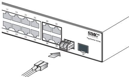
Figure 4-3 Making Fiber Port Connections
