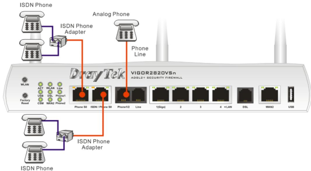
Yet, if the user configures ISDN / Phone S0 as TE Mode in **VoIP>> Phone Settings**, the **green** LED will light on to indicate **ISDN-TE** is selected. Then, the port is specified for ISDN line only. Refer to the following figure for reference.
