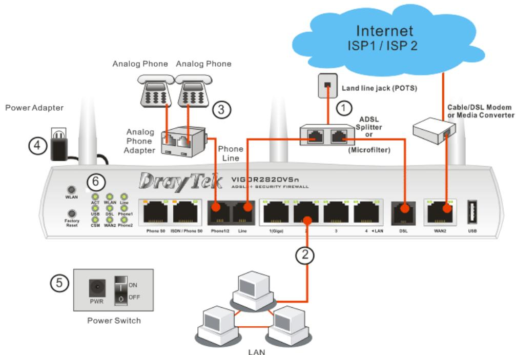
**Caution:** Each of the Phone ports can be connected to an analog phone only. Do not connect the phone ports to the telephone wall jack. Such connection might damage your router.
