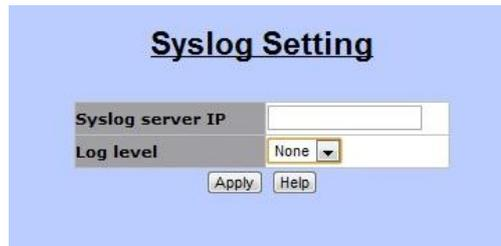
“Syslog” function is supported in this MINI IP DSLAM system. The system will send logs to a remote log system. In this system, three events will be reported to the remote log system: cold start, warm start and link change. The followings are necessary for connecting the remote syslog server.
