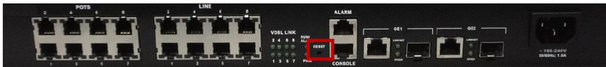
The reset buttons allows users to reboot the 8 Port Mini IP DSLAM or load the default settings.
