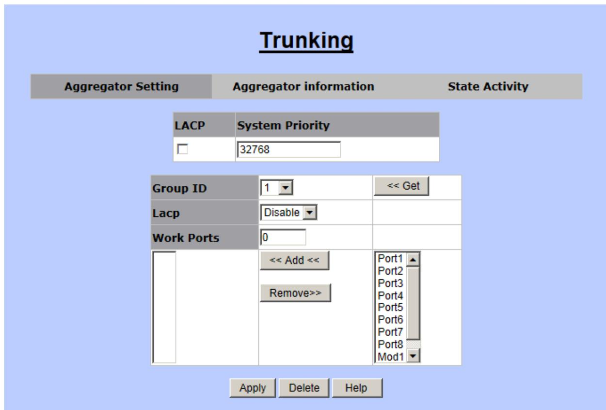
Trunking function allows users to combine several ports or connections together to create one single connection which has a higher and faster connection speed. “Trunking” is also called “Link Aggregation”. Two trunking techniques are available in this MINI IP DSLAM:
