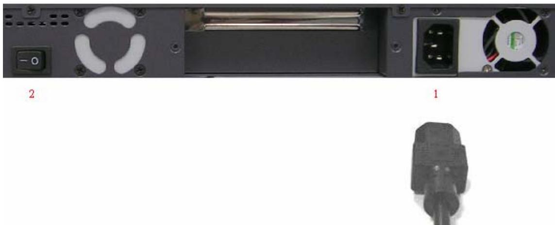
1. Connect the power cord to the power socket on the rear panel.
