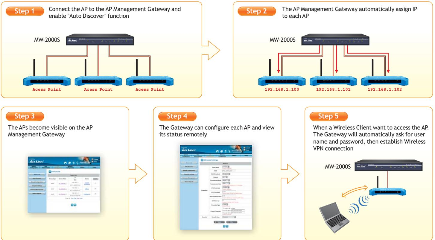
\* MW-2000S can work with both WL-5460AP e10.1 and WLA-5000AP v2.00e12 firmware. Please download the software from our website if you do not have the correct software installed in WL-5460AP or WLA-5000AP.
