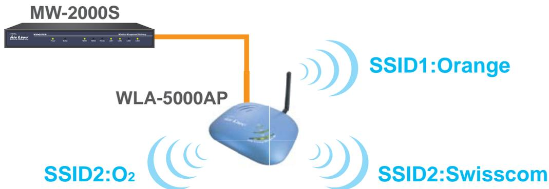
Deploy MW-2000S and several WLA-5000APs to construct the wireless environment, a specific work group can connect to their own SSID and access their own resource, even the user may not stay at the same place.
