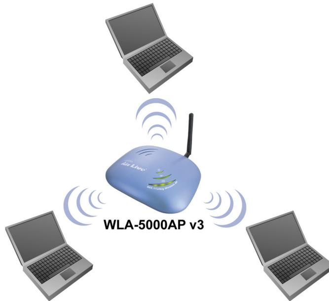
The WLA-5000AP v3 further provides bridging functions between the wireless network and the wired LAN network.
