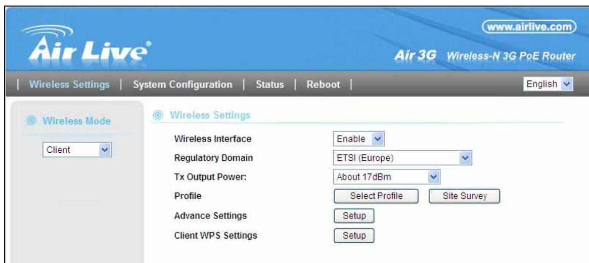
The screenshot shows the Air Live web interface for the Air 3G Wireless-N 3G PoE Router. The page title is "Air Live" and the URL is "www.airlive.com". The navigation menu includes "Wireless Settings", "System Configuration", "Status", and "Reboot". The "Wireless Settings" page is active, showing a "Wireless Mode" dropdown menu set to "Client". The "Wireless Settings" section includes the following options:
