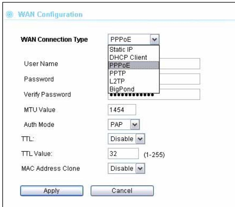
The screenshot shows the 'WAN Configuration' window. It includes a dropdown menu for 'WAN Connection Type' with options: PPPoE (selected), Static IP, DHCP Client, PPPoE, PPTP, L2TP, and BigPond. Other fields include: User Name, Password, Verify Password, MTU Value (1454), Auth Mode (PAP), TTL (Disable), TTL Value (32, range 1-255), and MAC Address Clone (Disable). 'Apply' and 'Cancel' buttons are at the bottom.
