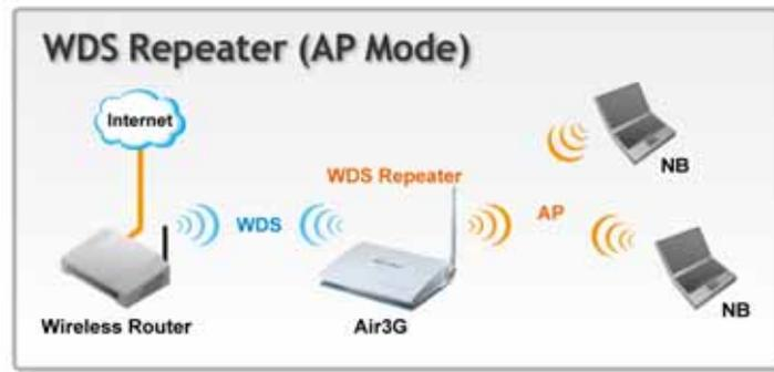
This is known as WDS Repeater function. Enable this setting to allow remote WDS equipped AP to extend the wireless signal of Air3G. Up to 4 WDS repeaters can be connect with Air3G. WDS works by entering the wireless MAC addresses (also known as BSSID) of remote Access Points.
