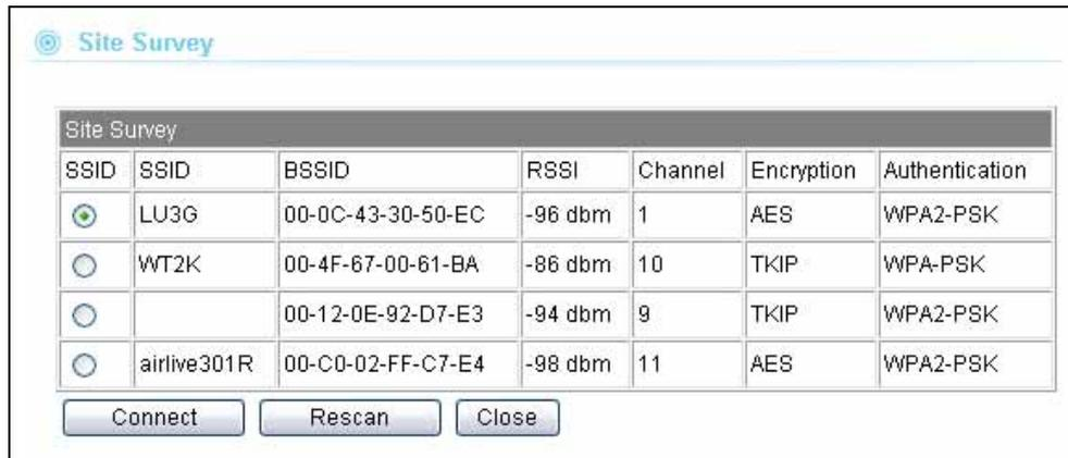
You can now select the SSID you want to connect with, then press the “Connect” button. If encryption key is required, the AP will prompt you to enter the encryption information.
