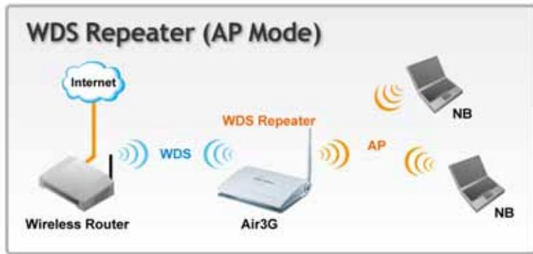
This is known as WDS Repeater function. In AP mode, the Air3G will repeat the wireless signal of remote AP/Router. Up to 4 WDS repeaters can be connect with Air3G. WDS works by entering the wireless MAC addresses (also known as BSSID) of remote Access Points.
