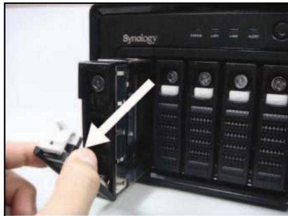
3. Attach the SATA hard disk to the hard disk tray and use 4 screws to fix the hard disk.
