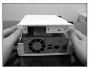
4. Place the hard disk inside the HDD bay.
