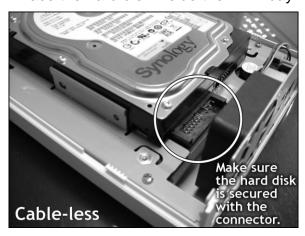
5. Fix the hard disk with the 4 HDD screws provided.
