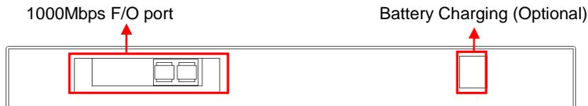
**Figure 8.** Rear Panel for 8-Port 10/100/1000Base-T plus 1-Port 1000Base-X or 100/1000Base-X Uplink Ethernet Managed Switch with Battery Charging Module (metal housing)
