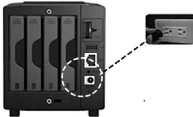
2. Use the LAN cable to connect the server to your switch/router/hub.
